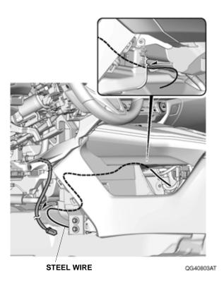
45. Attach the steel wire to the door sill trim harness with electrical tape.
