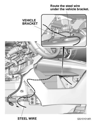
38. Attach the steel wire to the door sill trim harness with electrical tape.
