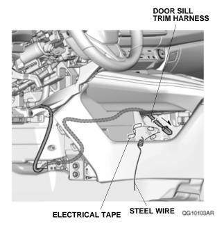
40. Remove the steel wire from the door sill trim harness.
