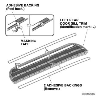
77. Remove the two adhesive backings.
