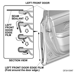
Using a shop towel, wipe the excess 3M protective tape application solution from the left front door edge film. Allow the left front door edge film to thoroughly dry.
