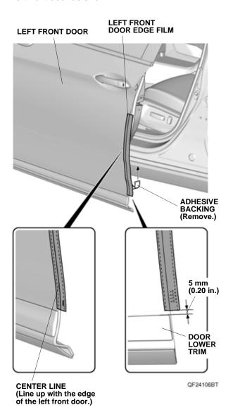
Line up the center line on the left front door edge film with the edge of the left front door. While applying light pressure, carefully remove the adhesive backing and attach the left front door edge film to the left front door. 8. Insert the applicator into the soft sleeve. Starting from the top and working downward, use the soft sleeve to smooth the left front door edge film. Move the soft sleeve in one direction only.
