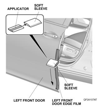
9. Slowly remove the protective film from the left front door edge film.
