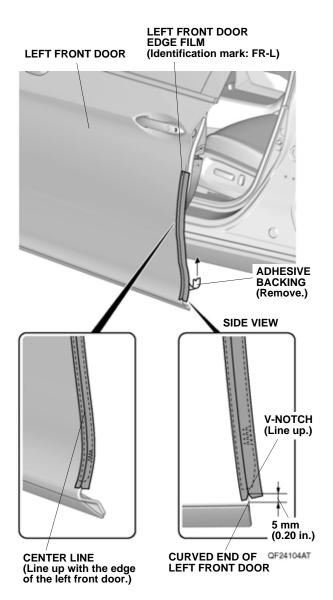
4. Line up the center line on the left front door edge film with the edge of the left front door. While applying light pressure, carefully remove the adhesive backing, and attach the left front door edge film to the left front door. Go to step 8.
