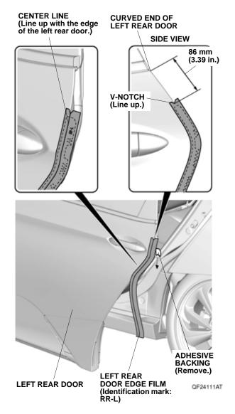
13. Line up the center line on the left rear door edge film with the edge of the left rear door. While applying light pressure, carefully remove the adhesive backing, and attach the left rear door edge film to the left rear door.
