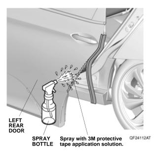
15. Line up the center line on the left rear door edge film with the edge of the left rear door. While applying light pressure, carefully remove the adhesive backing and attach the left rear door edge film to the left rear door.
