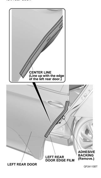
Starting from the top and working downward, use the soft sleeve to smooth the left rear door edge film. Move the soft sleeve in one direction only.
