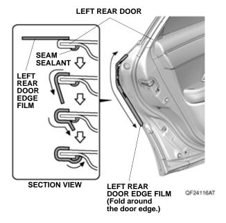
Using a shop towel, wipe the excess 3M protective tape application solution from the left rear door edge film. Allow the left rear door edge film to thoroughly dry.
