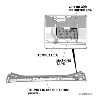
13. Using a pushpin, pierce the trunk lid spoiler trim through the 11 holes in template A. Remove template A.
