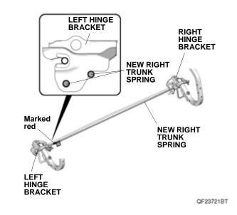
37. Install the center clip to the new right trunk spring.
