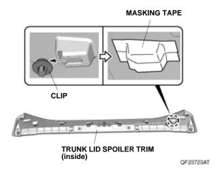
12. Place template A on the left side of the trunk lid spoiler trim and line up the template A with the trunk lid spoiler trim as shown. Tape the template A to the trunk lid spoiler trim with masking tape.
