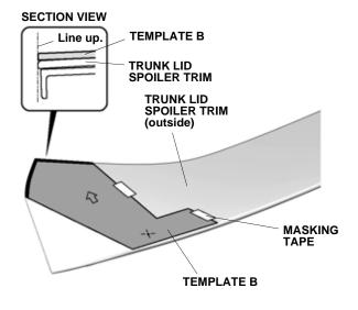
19. Apply masking tape to the trunk lid spoiler trim as shown.
