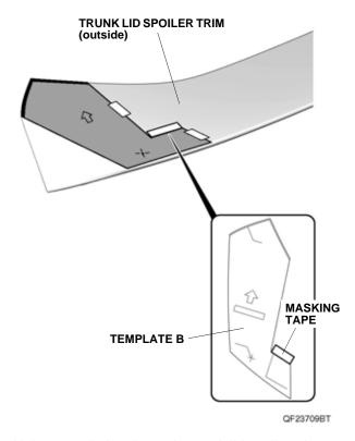
Using a pushpin, pierce the trunk lid spoiler trim through the one hole in template B. Remove template B.
