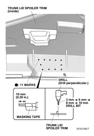
15. Using an air saw, cut out the trunk lid spoiler trim as shown. Remove any burrs.
