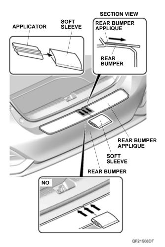
7. Starting from the front and working rearward, use the soft sleeve to smooth out the center of the upper section on the rear bumper applique. Move the soft sleeve in one direction only. If you see an air bubble, stop and gently peel up that section to work out the bubble. Work slowly and keep pressure against the
