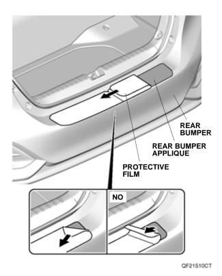
Repeat step 7 at the center of the lower section on the rear bumper applique.
