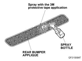
Line up the V-notch on the rear bumper applique with the trunk lid anchor. Line up the edge of the rear bumper applique along the end of the curved surface as shown. Smooth the rear bumper applique against the rear bumper.
