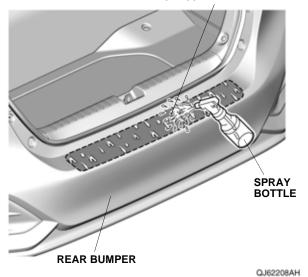
3. Remove the adhesive backing from the side of the rear bumper applique with the 3M mark.
