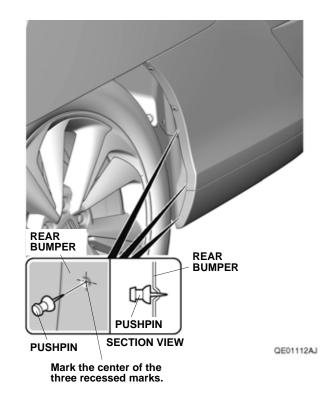
16. Install the three spring nuts on the rear bumper. Make sure to install the spring nuts in the correct position and orientation.
