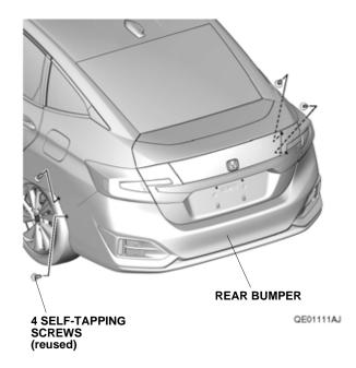
15. Locate the three recessed marks. Using a pushpin, pierce the rear bumper at the three recessed marks.
