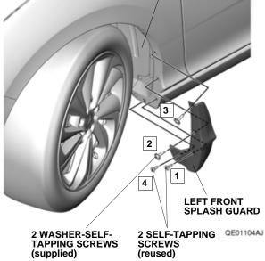
5. Turn the steering wheel fully clockwise, and repeat steps 2 through 4 to install the right front splash guard.
