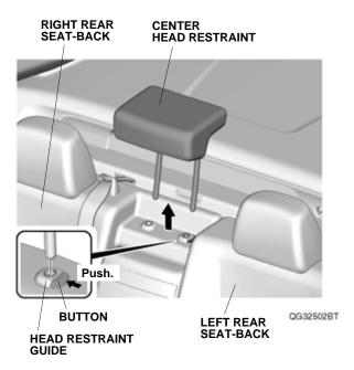
2. Install the head restraint cover on the center head restraint.
