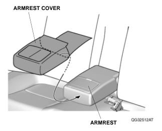
14. Pull out the armrest cover between the armrest and right rear seat-back, and secure the fasteners to each other as shown.
