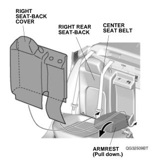
11. Fold the right rear seat-back forward, and secure the fasteners to the right rear seat-back.
