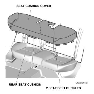
16. Secure the fasteners to the rear seat cushion, and insert the tabs under the rear seat cushion.
