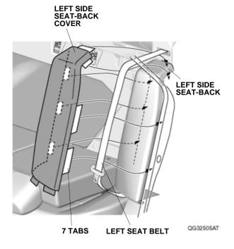
6. Insert the bottom tabs under the left side seat-back.
