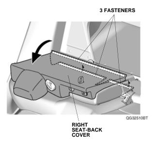
12. Tuck the right seat-back cover under each head restraint guide as shown.
