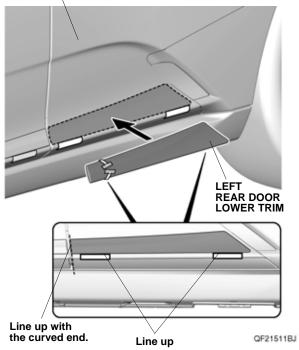
11. While applying light pressure against the left rear door lower trim, carefully remove the taped adhesive backings.
