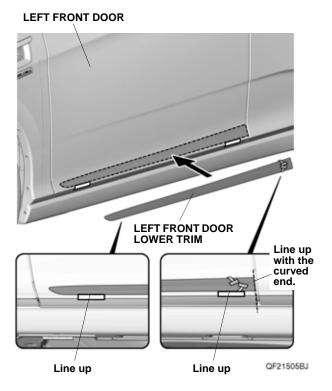
5. While applying light pressure against the left front door lower trim, carefully remove the taped adhesive backings.
