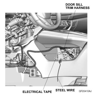
Remove the steel wire from the door sill trim harness.
