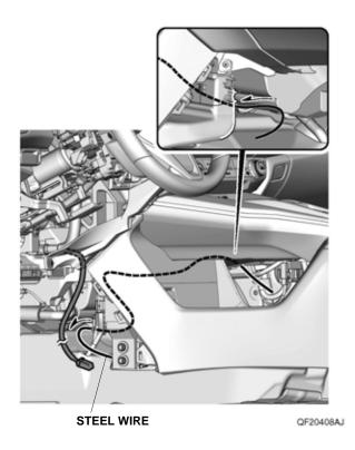
30. Attach the steel wire to the door sill trim harness with electrical tape.
