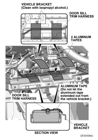
27. Secure the door sill trim harness to the vehicle bracket with two pieces of aluminum tape.
