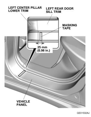
76. Peel back the end of one adhesive backing on the left rear door sill trim, and attach it to the front of the trim with masking tape.
