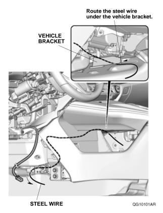
38. Attach the steel wire to the door sill trim harness with electrical tape.
