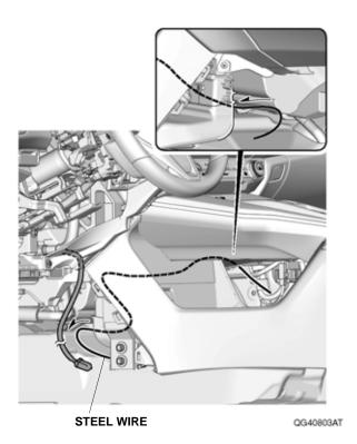
45. Attach the steel wire to the door sill trim harness with electrical tape.
