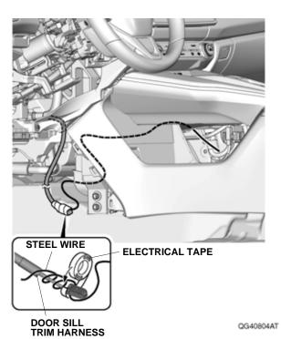
46. Pull the steel wire to route the door sill trim harness.
