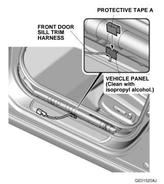
62. Attach one piece of protective tape A to the vehicle panel as shown.
