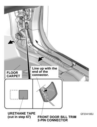
72. Plug the door sill trim harness 2-pin connector into the front door sill trim 2-pin connector.
