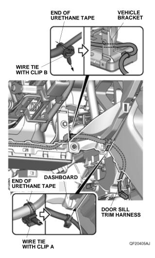
25. Secure the door sill trim harness to the dashboard with one wire tie with clip A.
