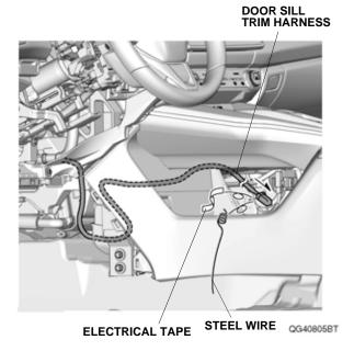
47. Remove the steel wire from the door sill trim harness.
