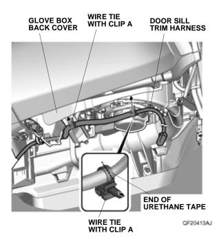
53. Using scissors, cut the protective tape as shown.
