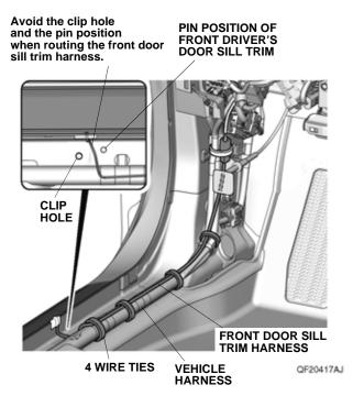
71. Attach one piece of the urethane tape around the front door sill trim 2-pin connector.
