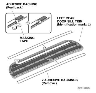
77. Remove the two adhesive backings.
