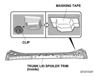
12. Place template A on the left side of the trunk lid spoiler trim and line up the template A with the trunk lid spoiler trim as shown. Tape the template A to the trunk lid spoiler trim with masking tape.
