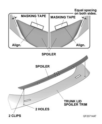
27. While applying light pressure against the spoiler, carefully remove the adhesive backings as shown.
