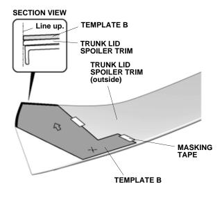
19. Apply masking tape to the trunk lid spoiler trim as shown.
