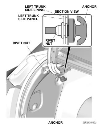
26. Install three small washers and one bolt into one anchor.
