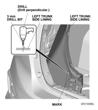
22. Enlarge the 3 mm hole to 13 mm using a 13 mm hole saw. Be careful not to crease the left trunk side lining.
