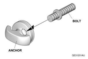
25. Install one anchor into the rivet nut.
