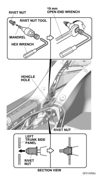
18. Loosely install the bolt, large washer, and flange nut into the rivet nut.
