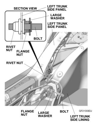
19. Mark the left trunk side lining with a felt-tip pen as shown.
