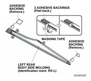
10. Line up the left rear body side molding with the rear template, and install the left rear body side molding on the left rear door.
