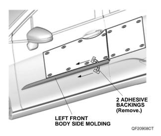
8. Using the rubber roller, apply firm pressure while rolling, especially at the ends, to set the adhesive.
