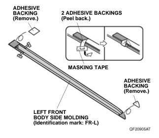
6. Line up the left front body side molding with the front template, and install the left front body side molding on the left front door.
