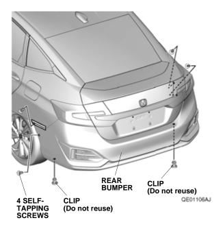
8. Release the three retaining tabs on each side.
