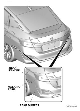
7. Remove the four self-tapping screws and two clips.
