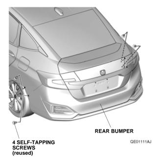
15. Locate the three recessed marks. Using a pushpin, pierce the rear bumper at the three recessed marks.
