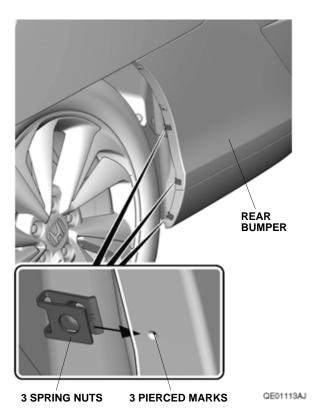
17. Secure the left rear splash guard with three selftapping screws and one clip in the order shown below.
