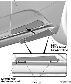
While applying light pressure against the left rear door lower trim, carefully remove the taped adhesive backings.
