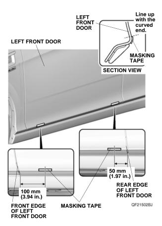
Using an alcohol swab, thoroughly clean the left front door where the left front door lower trim will attach.
