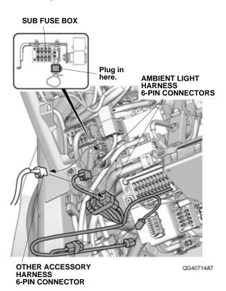
32. Route the ambient light harness as shown. Secure the ambient light harness 10-pin connector to the vehicle harness with one wire tie.
