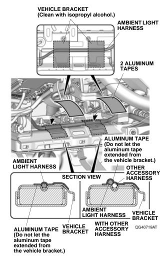
41. Secure the ambient light harness to the vehicle bracket with two pieces of aluminum tape.
