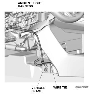
51. Secure the ambient light harness to the glove box back cover with two wire ties with clip A. If another accessory harness is already secured to the glove box back cover, secure the ambient light harness to the other accessory harness with two wire ties with clip A.
