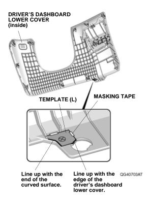
15. Using a pushpin, pierce the center of the mark on the template.
