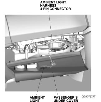
53. Plug the ambient light harness 4-pin connector into the ambient light, and install the passenger's under cover.
