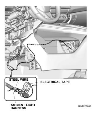
45. Pull the steel wire to route the ambient light harness.
