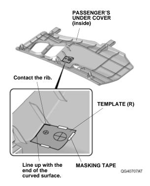
21. Using a pushpin, pierce the center of the two marks on the template.
