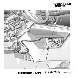
46. Remove the steel wire from the ambient light harness.
