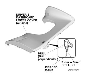
18. Using a file, remove any burrs from the hole.
