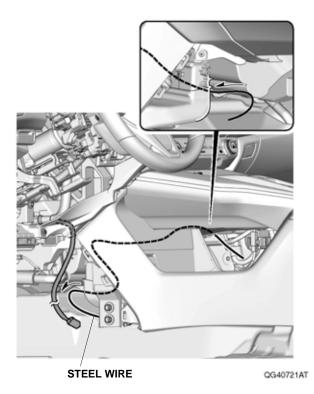
44. Attach the steel wire to the ambient light harness with electrical tape.
