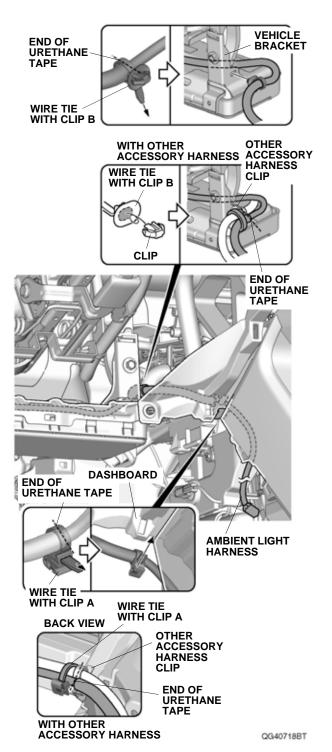
39. Secure the ambient light harness to the dashboard with one wire tie with clip A. If another accessory harness is already secured to the dashboard, secure the ambient light harness to the other accessory harness with one wire tie with clip A. 40. Using isopropyl alcohol on a shop towel, thoroughly clean the vehicle bracket where the aluminum tape will attach.
