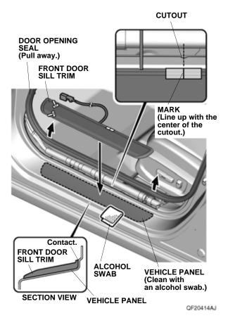
58. Pull away the door opening seal, and line up the mark on the front door sill trim with the center of the cutout of the vehicle panel.
