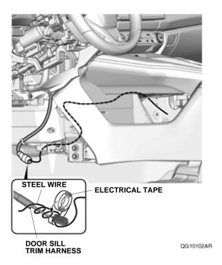
Pull the steel wire to route the door sill trim harness.
