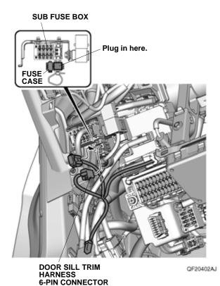
20. Attach the door sill trim harness fuse case to the vehicle 6-pin connector.
