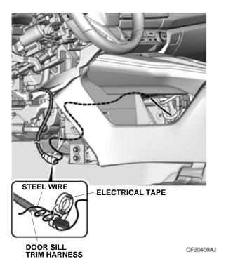
31. Pull the steel wire to route the door sill trim harness.
