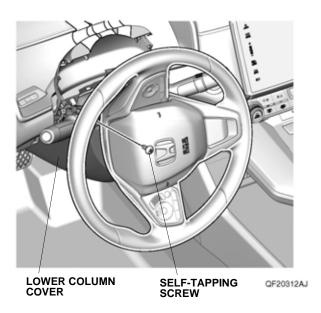
14. Turn the steering wheel 180° clockwise, and remove the self-tapping screw from the lower column cover.
