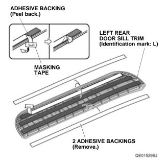
77. Remove the two adhesive backings.
