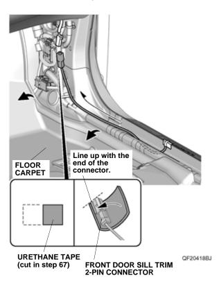
72. Plug the door sill trim harness 2-pin connector into the front door sill trim 2-pin connector.
