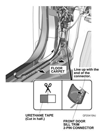
68. Plug the door sill trim harness 2-pin connector into the front door sill trim 2-pin connector.
