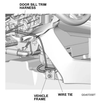
52. Secure the door sill trim harness to the glove box back cover with two wire ties with clip A.
