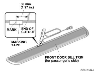
55. Peel back the ends of two adhesive backings on the front door sill trim, and attach them to the front of the trim with masking tape.
