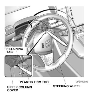
11. Turn the steering wheel 180° counterclockwise. Using a plastic trim tool, release one retaining tab.
