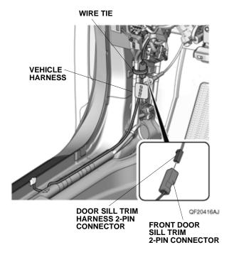
69. Secure the 2-pin connectors to the vehicle harness with one wire tie.
