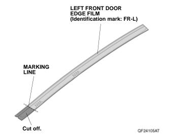
6. Open the left front door. Peel back about 50 mm (1.97 in.) of adhesive backing from the left front door edge film. Line up the left front door edge film on the left front door as shown.
