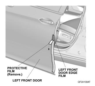
10. Starting from the center and working outward, use your fingers to fold the left front door edge film around the edge of the left front door as shown. Move your fingers in one direction only. Attach the left front door edge film over the seam sealant. Do not trim or damage the seam sealant.
