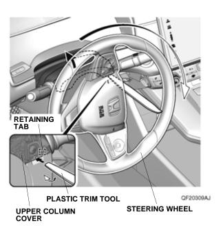
7. Turn the steering wheel 180° counterclockwise. Using a plastic trim tool, release one retaining tab.
