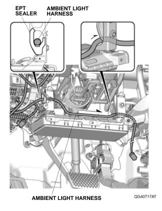
38. Secure the ambient light harness to the vehicle bracket with one wire tie with clip B. If another accessory harness is already secured to the vehicle bracket, secure the ambient light harness to the other accessory harness with one wire tie with clip B.
