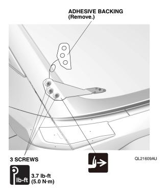
28. Temporarily attach the adhesive backings.
