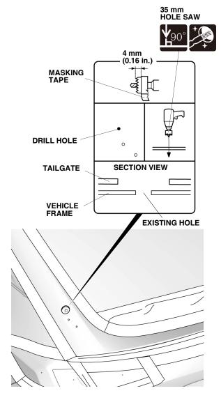
14. Attach masking tape to protect the vehicle.
