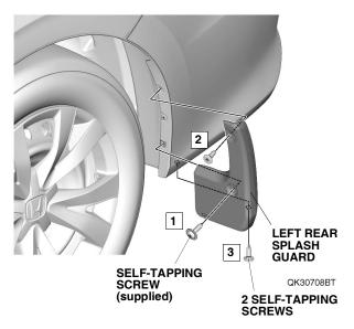
9. Turn the steering wheel fully clockwise, and repeat the same procedures on the other side.
