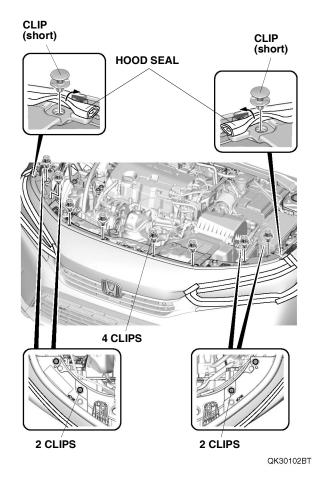
4. Remove the self-tapping screws, clips, and bolts.
