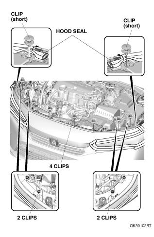
4. Remove the self-tapping screws, clips, and bolts.
