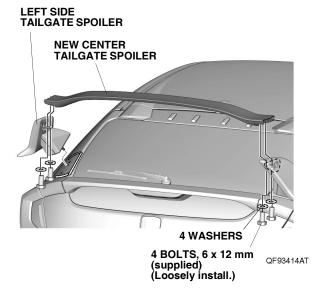
15. Open the tailgate, and secure the left side tailgate spoiler with two 6 x 65 mm bolts.
