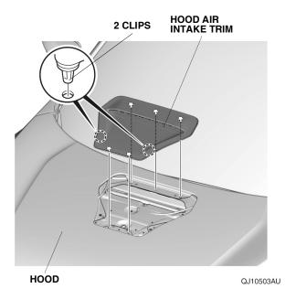
Secure the hood air intake trim to the hood with five nuts. Torque the nuts to 6.9 lb-ft (9.4 N·m).
