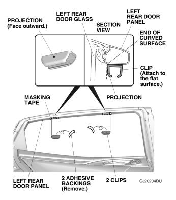
5. Remove the adhesive backings. Then, line up each clip as shown and attach the clips to the door lining. NOTE: Press down and hold each clip in place for 30 seconds to allow the adhesive to set.
