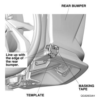
6. Using a felt-tip pen, mark the left rear inner fender along the template.
