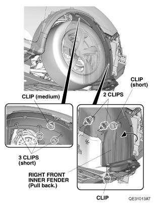
15. Remove the eight clips from the left front inner fender and pull it back as shown.
