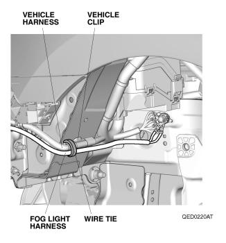
48. Plug two fog light harness 2-pin connectors into each fog light, then with the help of an assistant, install the front bumper.
