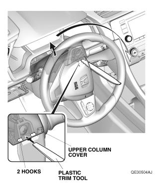
7. Turn the steering wheel 180° counterclockwise. Using a plastic trim tool, release the two hooks.
