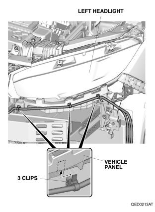
41. Secure the three clips on the fog light harness to the vehicle panel as shown.
