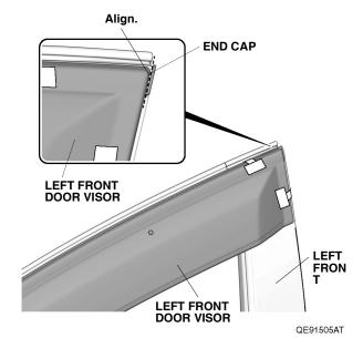
While applying light pressure against the left front door visor, carefully remove the adhesive backings in the order shown. Make sure to push up on the brackets while removing the adhesive backings.
