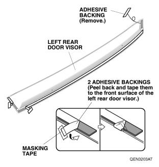
16. Remove the adhesive backing.
