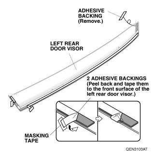
16. Remove the adhesive backing.
