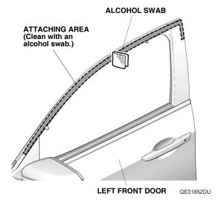
5. Peel back the adhesive backing from each adhesive tape and tape the ends to the front surface of the left front door visor with masking tape.
