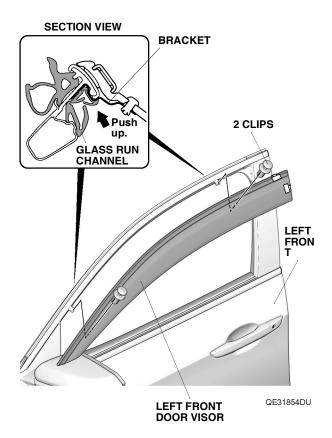
7. Secure the left front door visor to the two brackets with two clips. Make sure to push up on the brackets while installing the two clips.
