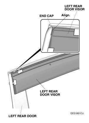
20. While applying light pressure against the left rear door visor, carefully remove the taped adhesive backings in the order shown. Make sure to push up on the brackets while removing the adhesive backings.
