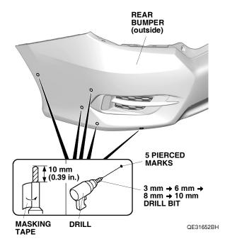
6. Using a file, remove any burrs from the holes.
