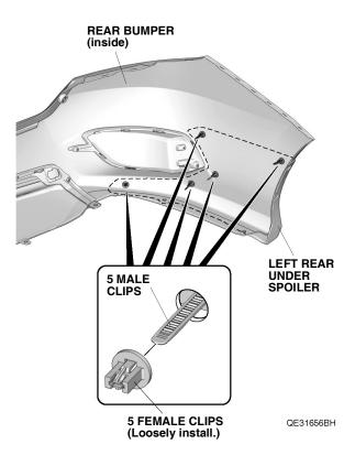
11. Remove the three adhesive backings in the order shown. Press the left rear under spoiler firmly against the rear bumper with the palm of your hand to adhere the left rear under spoiler.
