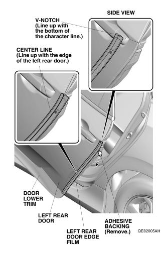
19. Line up the center line on the left rear door edge film with the edge of the left rear door. While applying light pressure, carefully remove the adhesive backing and attach the left rear door edge film to the left rear door.
