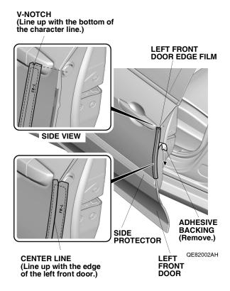
7. Line up the center line on the upper part of left front door edge film with the edge of the left front door. While applying light pressure, carefully remove the adhesive backing and attach the upper part of the left front door edge film to the left front door.
