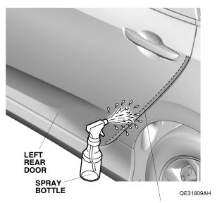
Spray with 3M protective tape application solution.
