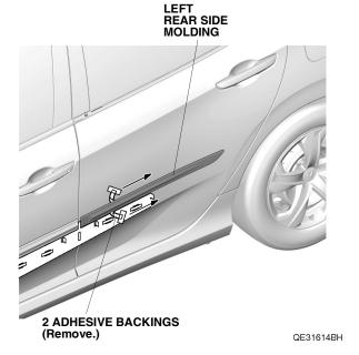
12. Using a rubber roller, apply firm pressure while rolling, especially at the ends, to set the adhesive.
