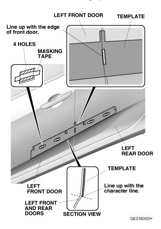
3. Using an alcohol swab, thoroughly clean the left front door where the left front side molding will attach.
