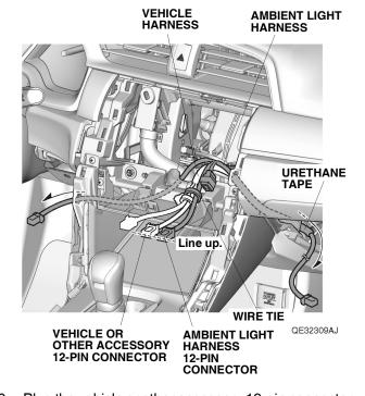
29. Plug the vehicle or other accessory 12-pin connector into the ambient light harness 12-pin connector, and secure the ambient light harness to the vehicle harness with one wire tie.
