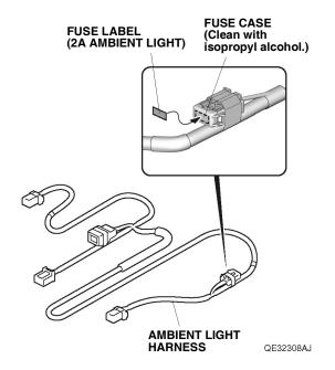
27. Attach the fuse label to the ambient light harness fuse case.
