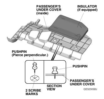
21. While wearing eye protection, drill the pierced mark with a 3 mm drill bit, then finish with a 5 mm drill bit as shown.
