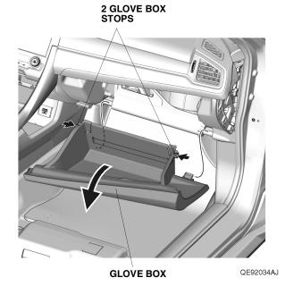
5. Remove the glove box cover, and unplug the vehicle connector, if equipped.
