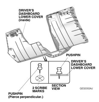
16. While wearing eye protection, drill the pierced mark with a 3 mm drill bit, then finish with a 5 mm drill bit as shown.
