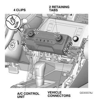
14. Remove the audio unit, and unplug the vehicle connectors.
