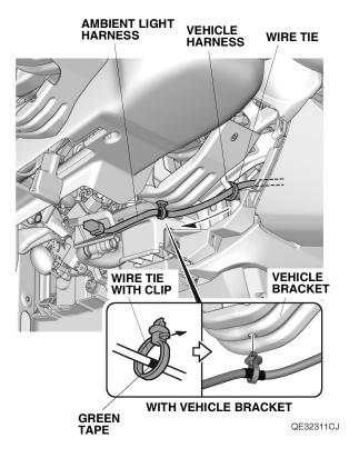
31. Secure the ambient light harness to the vehicle harness with one wire tie.
