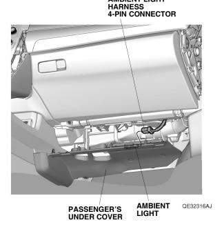
39. Plug the ambient light harness 4-pin connector into the ambient light, and install the passenger's under cover.
