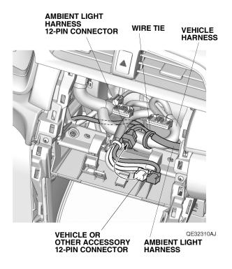
30. If equipped with the vehicle bracket, secure the green tape on the ambient light harness to the vehicle bracket with one wire tie with clip.
