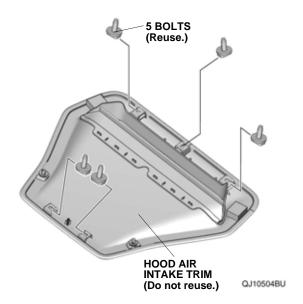
4. Install the five bolts to the new hood air intake trim. NOTE: Make sure the bolts are fully inserted into the clip base for proper installation.
