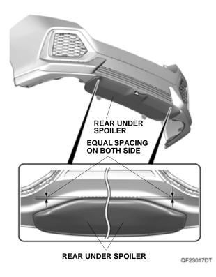
15. Remove the adhesive backing as shown. Press the rear under spoiler firmly against the rear bumper with the palms of your hands.
