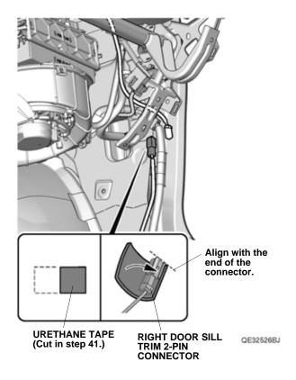
46. Plug the door sill trim harness 2-pin connector into the right door sill trim 2-pin connector.
