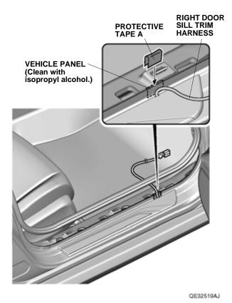
32. Install the protective clip to the protective tape A.
