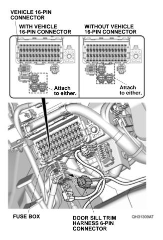
15. Attach the door sill trim harness fuse case to the vehicle connector.
