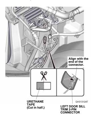
42. Plug the door sill trim harness 2-pin connector into the left door sill trim 2-pin connector.
