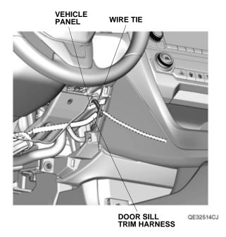
22. Route the door sill trim harness as shown. Secure the door sill trim harness to the vehicle harness with four wire ties.
