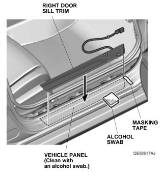
28. Line up the right door sill trim with the masking tape as shown.
