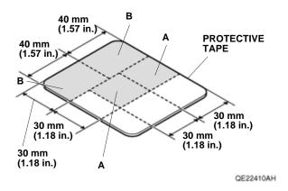
24. Attach masking tape to the vehicle panel as shown.
