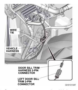
43. Secure the 2-pin connectors to the vehicle harness with one wire tie.
