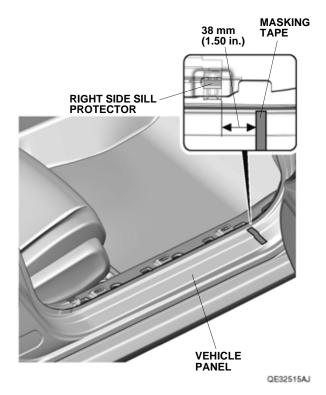
25. Peel back the ends of two adhesive backings on the right door sill trim, and attach them to the front of the trim with masking tape.
