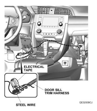
20. Route the door sill trim harness as shown, and remove the electrical tape and steel wire.
