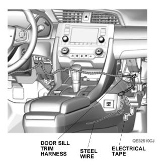
21. Secure the door sill trim harness to the vehicle panel with one wire tie.
