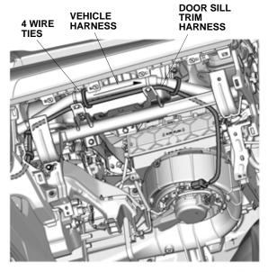
23. Using scissors, cut the protective tape as shown.
