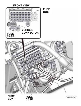
Route the door sill trim harness as shown. Secure the door sill trim harness to the vehicle harness and bracket with four wire ties.
