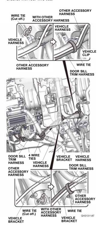
17. Secure the door sill trim harness to the vehicle duct with two wire ties.
