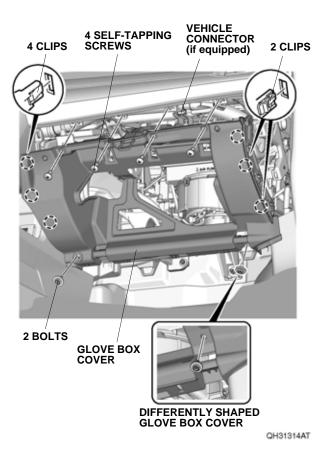
8. Remove the driver's dashboard lower cover, unplug the vehicle connectors and aspirator hose.
