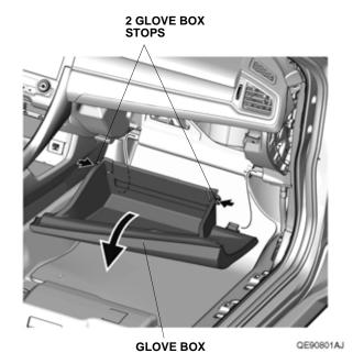
7. Remove the glove box cover, and unplug the vehicle connector, if equipped.
