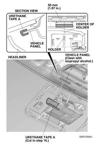
Attach urethane tape A to the vehicle panel.
