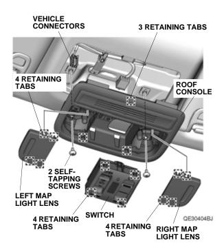
Without Moonroof and With Ambient light: Remove the roof console, and unplug the vehicle connectors.
