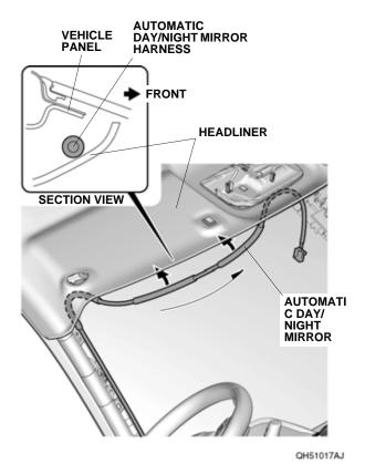
33. Line up the end of the urethane tape on the automatic day/night mirror harness with the vehicle bracket, and secure the automatic day/night mirror harness to the vehicle harness with one wire tie as shown.
