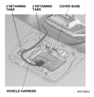
22. Wrap the urethane tape to the vehicle connector and vehicle harness as shown.
