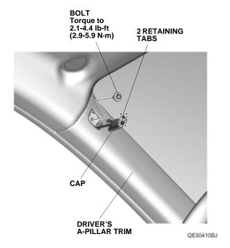
11. Pull away the door opening seal, and remove the driver's A-pillar trim.
