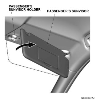
7. Remove the passenger's sunvisor holder by rotating it 90° counterclockwise.
