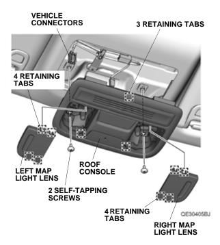
Without Moonroof and Ambient light: Remove the roof console, and unplug the vehicle connectors.
