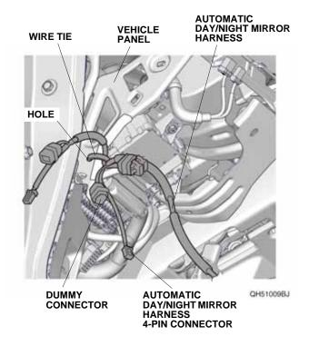
If the vehicle is equipped with another accessory harness 4-pin connector, go to step 26; otherwise, continue with step 25.
