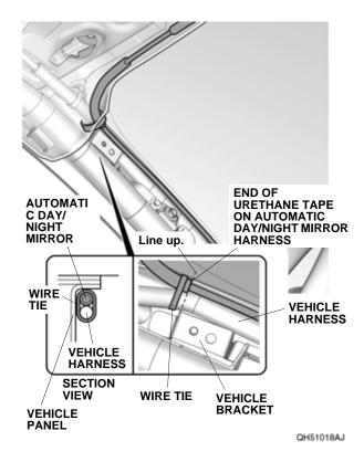
34. Using isopropyl alcohol on a shop towel, thoroughly clean the vehicle panel where the aluminum tape will attach.
