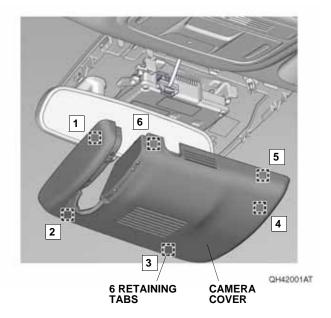
4. Loosen the Torx screw, and remove the rearview mirror from the mirror mount, and unplug the vehicle connector (if equipped).
