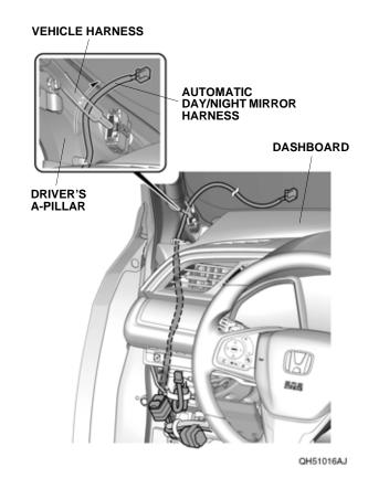
32. Route the automatic day/night mirror harness along the driver's A-pillar. Gently pull back the headliner, and tuck the automatic day/night mirror harness behind the headliner.
