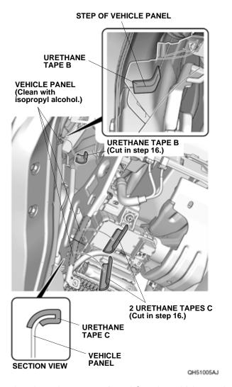
20. Attach urethane tapes B and C to the vehicle panel.
