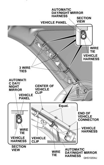
37. Secure the automatic day/night mirror harness to the vehicle panel with two wire ties.
