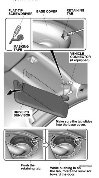
9. Remove the driver's sunvisor holder by rotating it 90° counterclockwise.
