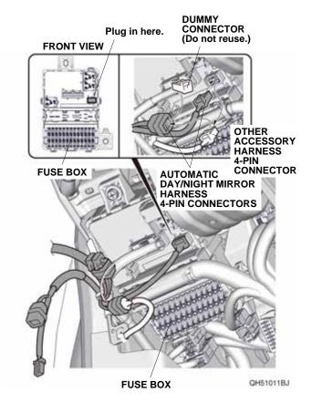
27. Secure the automatic day/night mirror harness to the vehicle harness with one wire tie.
