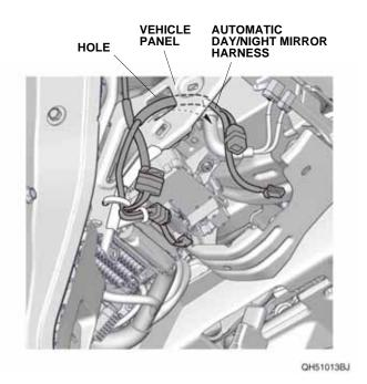
Plug the vehicle 4-pin connector (VSA OFF switch) into the automatic day/night mirror harness 4-pin connector.
