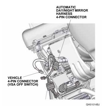
30. Line up the branch of the automatic day/night mirror harness with the vehicle clip, and secure the automatic day/night mirror harness and 4-pin connectors to the vehicle harness with two wire ties.
