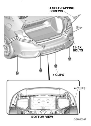
• With center muffler: Remove the two hex bolts, four clips, and four self-tapping screws.
