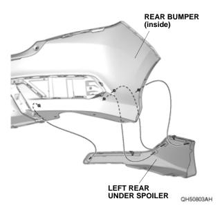
10. Loosely install the four female clips into each of the male clips.
