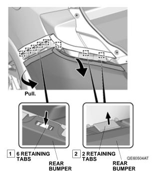
With the help of an assistant, remove the rear bumper. Place the rear bumper on a blanket to prevent damage.
