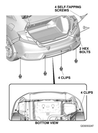
With dual mufflers: Remove the two hex bolts, four clips, and four self-tapping screws.
