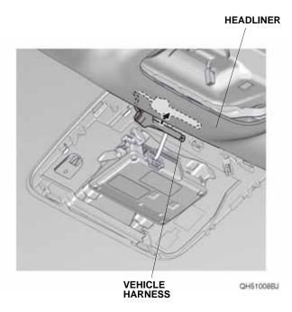
24. Secure the automatic day/night mirror harness to the vehicle panel with one wire tie as shown.
