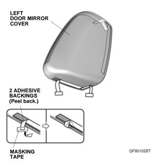
Using an alcohol wipe, thoroughly clean the left mirror housing upper cover where the left door mirror cover will attach.
