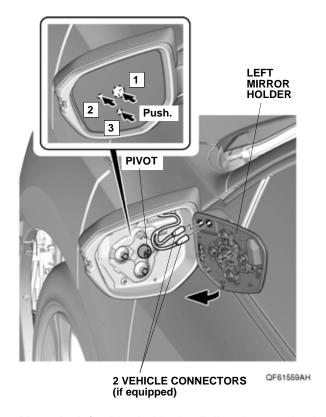
14. Move the left mirror holder in all directions to check if it is installed securely.
