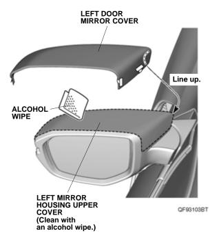
17. Line up the left door mirror cover with the left mirror housing upper cover as shown.
