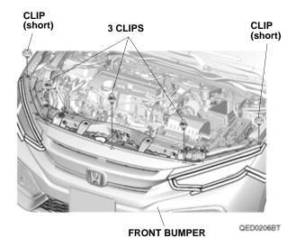
With the help of an assistant, remove the front bumper. Place the front bumper on a blanket to prevent damage.
