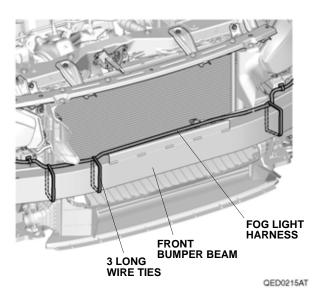
43. Join four long wire ties together as shown and secure the fog light harness to the front bumper beam with two joined long wire ties.
