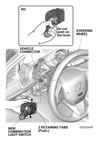
63. Plug the vehicle connector into the new combination light switch.
