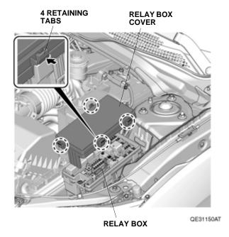
67. Using isopropyl alcohol on a shop towel, thoroughly clean the relay box cover where the fuse label will attach.
