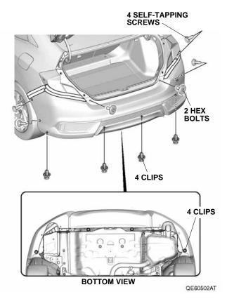
With dual muffler: Remove two hex bolts, four clips, and four self-tapping screws.
