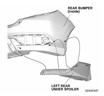
10. Loosely install four female clips into each of the male clips.
