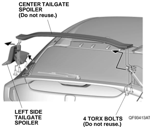
14. Loosely install the new center tailgate spoiler and left side tailgate spoiler as shown.
