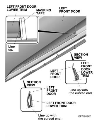
5. While applying light pressure against the left front door lower trim, carefully remove the taped adhesive backings.
