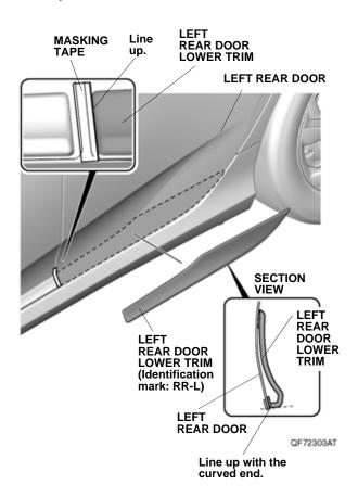
10. Apply masking tape to the left rear door as shown. Remove the left rear door lower trim.
