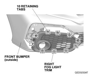
27. Install the right fog light trim to the front bumper with one clip. Go to step 34.
