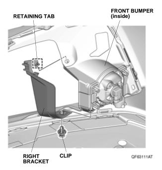
26. Install the right fog light trim to the front bumper with the 10 retaining tabs.
