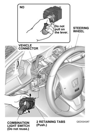
61. While pushing the two retaining tabs, slide the combination light switch out and remove it from the steering column.
