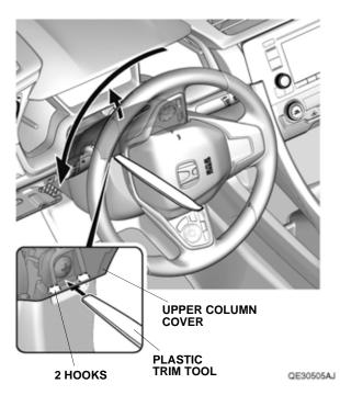
8. Release the upper column cover and secure it to the dashboard with masking tape.
