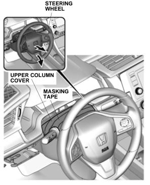
6. If necessary, connect the negative cable to the battery and set the power mode to ON. Turn the steering wheel 90° clockwise. Using a plastic trim tool, release the hooks.
