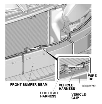
45. Line up the fog light harness with the vehicle clip and secure the fog light harness to the vehicle harness with one wire tie.
