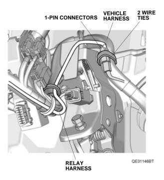
60. Unplug the vehicle connector from the combination light switch.
