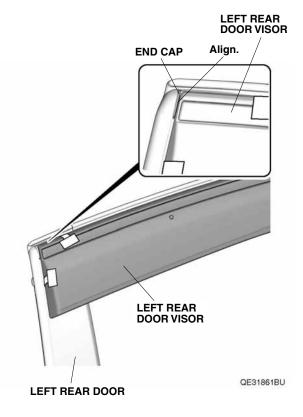
20. While applying light pressure against the left rear door visor, carefully remove the adhesive backings in the order shown. Make sure to push up on the brackets while removing the adhesive backings.
