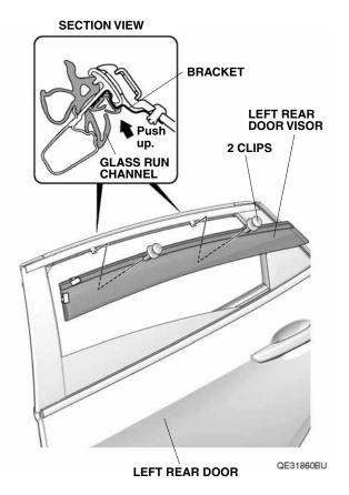
Secure the left rear door visor to the two brackets with two clips. Make sure to push up on the brackets while installing two clips.
