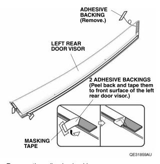
16. Remove the adhesive backing.
