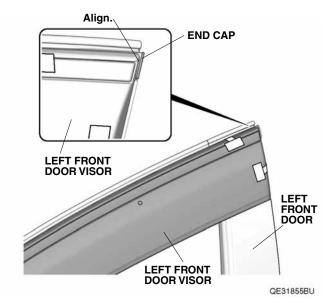
While applying light pressure against the left front door visor, carefully remove the adhesive backings in the order shown. Make sure to push up on the brackets while removing the adhesive backings.
