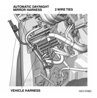
If the vehicle is equipped with another accessory harness 4-pin connector, go to step 22. If not, continue with step 21.
