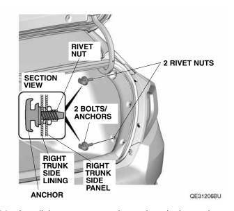
14. Install the cargo net on the anchors in the trunk.
