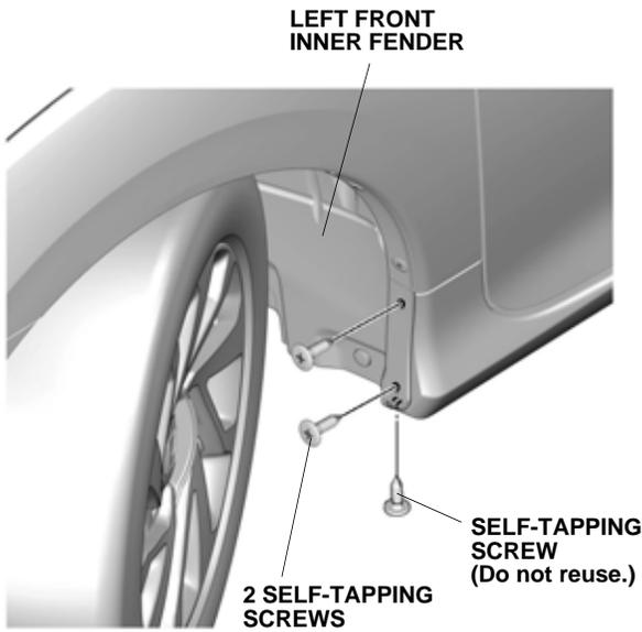
2. Remove three self-tapping screws from the left front inner fender.
