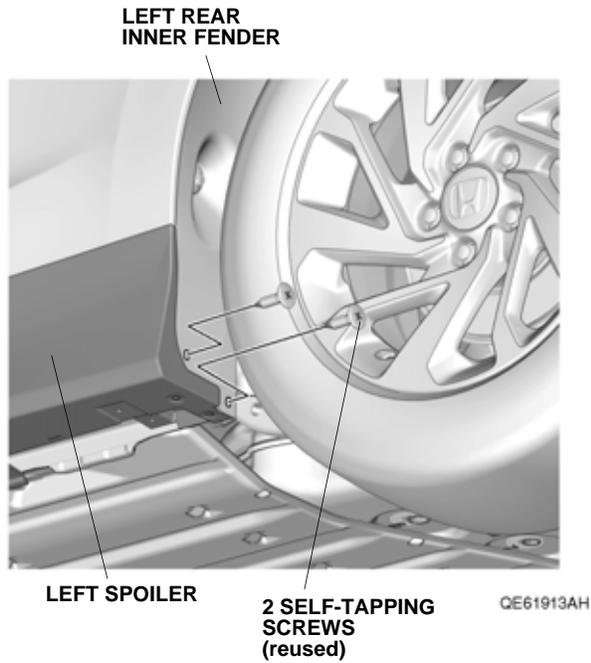
17. Turn the steering wheel fully clockwise, and repeat steps 2 through 16 on the right side of the vehicle.
