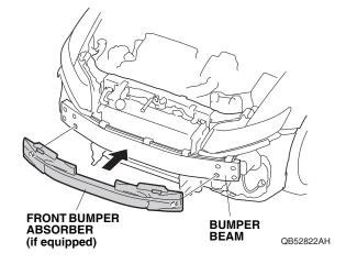
42. Plug the fog light harness 2-pin connector into each fog light, and with the help of an assistant, reinstall the front bumper.
