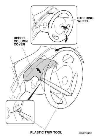
7. Using a plastic trim tool, release the lock tab as shown.
