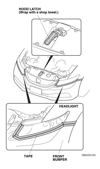
• Remove the 2 self-tapping screws, 10 clips, and 2 bolts.
