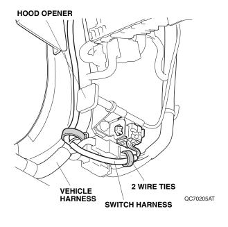
58. Secure the switch harness to the vehicle harness with two wire ties.
