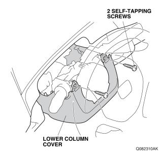
Remove the lower column cover (one self-tapping screw).
