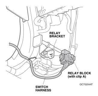
54. Plug the switch harness 4-pin connector and 6-pin connector into the fuse box. Go to step 57.
