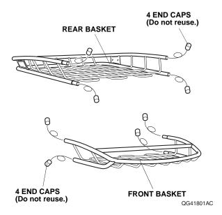
2. Attach the front and rear baskets to each other with 6 x 12 mm bolts and 12 mm washers. Torque the bolts to 2.2 lb-ft (3 N·m).
