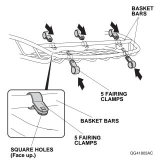
Remove the protection film from the basket fairing, and place it on top of the fairing clamps. Then, secure the basket fairing to the fairing clamps with carriage bolts B, 20 mm washers, and the fairing thumbwheels.
